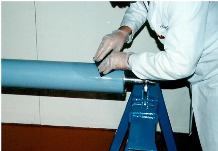
As the adhesive is pushed along the roll under the cover, it is probable that air will become entrapped. Such air must be pushed out of the cover towards the ends of the roller otherwise not only will it prevent bonding at that point but when the roller is heated in operation, the air will expand and cause appreciable bumps on the surface of the cover.
