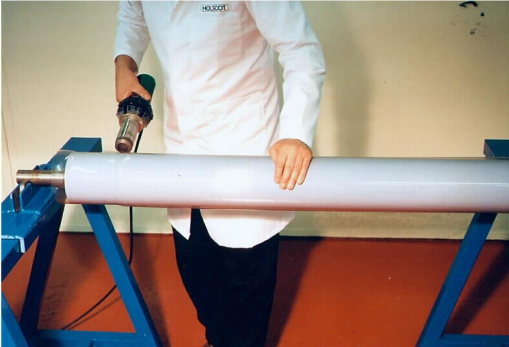
The surface of the roll to be covered must be smooth, clean and dry. The roll need not be machined or ground, but foreign materials such as grease, oil, dirt, loose scale, product build up, etc., must be removed. The roller should also be slightly above room temperature before the cover is installed. A warm roller is faster. This applies particularly to metal rollers which must be warmed before the sleeve is fitted.
