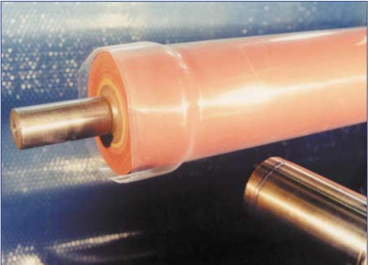
The Holscot range of heat shrinkable sleeves encompasses sizes from 12mm to 400mm as a seamless sleeve. Easily installed using a hot air gun, the most widespread use is as a non-stick surface for rollers in such industries as the paper, printing and textile industries.
