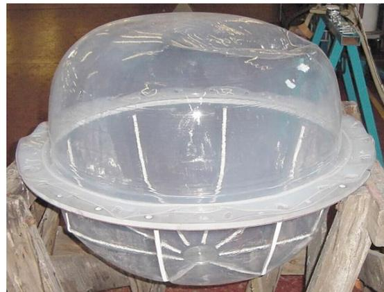
FEP, which is completely inert, was to be used instead of the rubber tank liner, which had been used previously. The FEP was specified to avoid contamination of the potable water.
