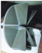
Photo 2 – Halar ECTFE coated agitator.
